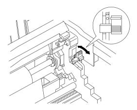
☐ Move the adjustment lever on the right side of the platen to one of its four settings. The adjustment lever position that is nearest to the back of the printer is Position 1 (minimum gap), while the position at the opposite extreme is Position 4 (maximum gap). Position 2, which is marked with a dot, is most suitable for single-sheet paper.
