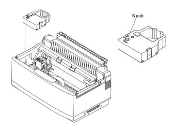
☐ If you have a color printer model, be sure to carefully position the ribbon between the print head and the print head shield as shown in the illustration.
