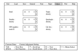
The above window is used to test and adjust the vertical alignment of the printer in each printing mode. You may never have to use the procedure described in this section, but after you have been using your printer for some time you may find that the dots of some graphics do not align correctly. For example, what should look like:
